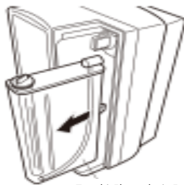
Tangki Electrolysis Enhancer
